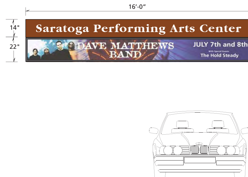
SPAC Signage at Route 50 Pedestrian Bridge Scale 1/4"=1'-0" • Combination designation header and marquee digital display mounted on Route 50 pedestrian bridge. • Dimensions shown are approximate and may be scaled proportionally.
