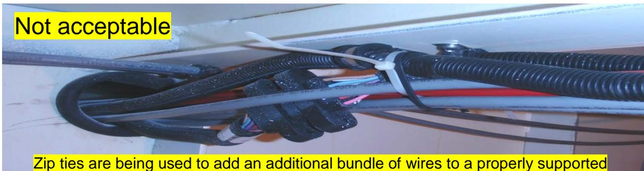
The use of house wire or speaker wire is not acceptable. Conductors shall be stranded, not solid, copper and must be labeled "marine" or "boat". For AC and especially for DC systems there are formulas you need to use when adding or replacing equipment on board. The Marine Services Bureau can assist you in determining the correct wire sizes.
